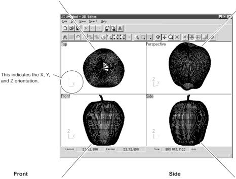
This is a view of the object seen from directly in front. You can move only in the X and Z directions; there is no movement in the Y-axis direction. Use this at times such as when you want an accurate view of movement along the Z axis.
